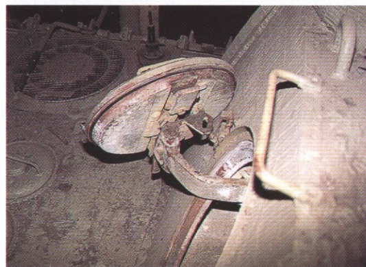
Inside detail shot of the escape/ammo loading hatch with hinge and securing bracket. Note the handhold on top of the turret above the hatch.
