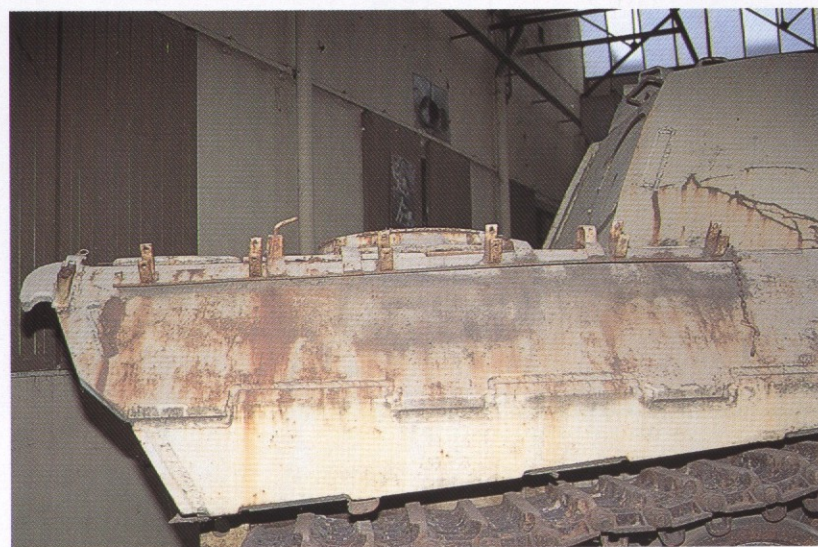
A view of the same area without the side skirts installed reveals the welding seams and the sloped bottom.
