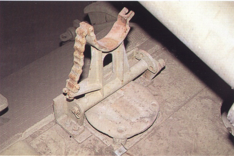
Gun tube travel lock with securing chain on the front upper hull.
