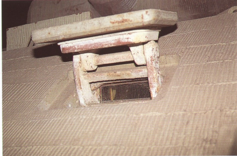
Driver's vision slot with protective hatch which can be opened or closed from inside the driver's compartment.
