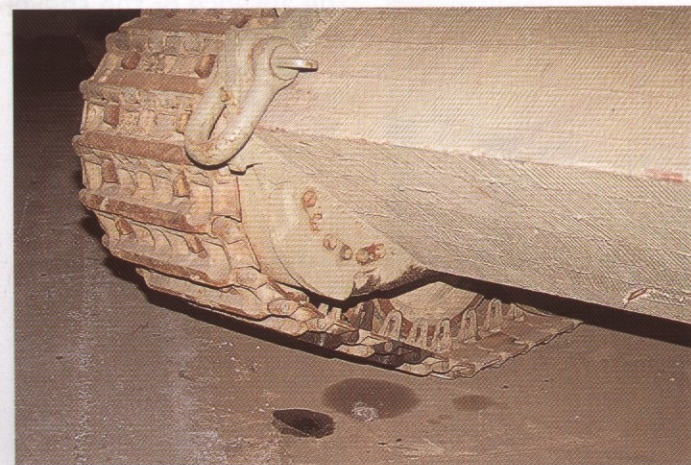
Closer look at the final drive gear housing. Note the application of the zimmeritt paste. At right can be seen the black out light, installed on port side only.
