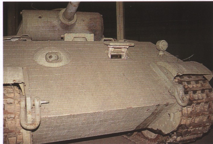
View on the frontal hull and front starboard side. Bottom hull plate is 60mm armor plate, sloped 56° from the vertical; upper hull armor plate is 80mm thick and sloped 55° from the vertical. Note the towing hooks next to the tracks.
