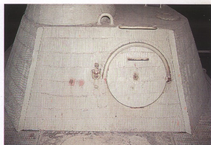
The rear turret escape hatch seen here in both open and closed position is also used for loading ammo. Similar to the sighting telescope port, the escape hatch has a rain deflection shield on the upper side. Note the 45mm armor plate on the side of the turret.
