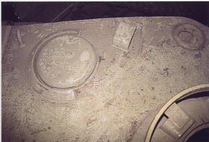
Upper turret detail with lifting hook, ventilator fan cover with protective side rim, loader's periscope cover and S-mine thrower port.
