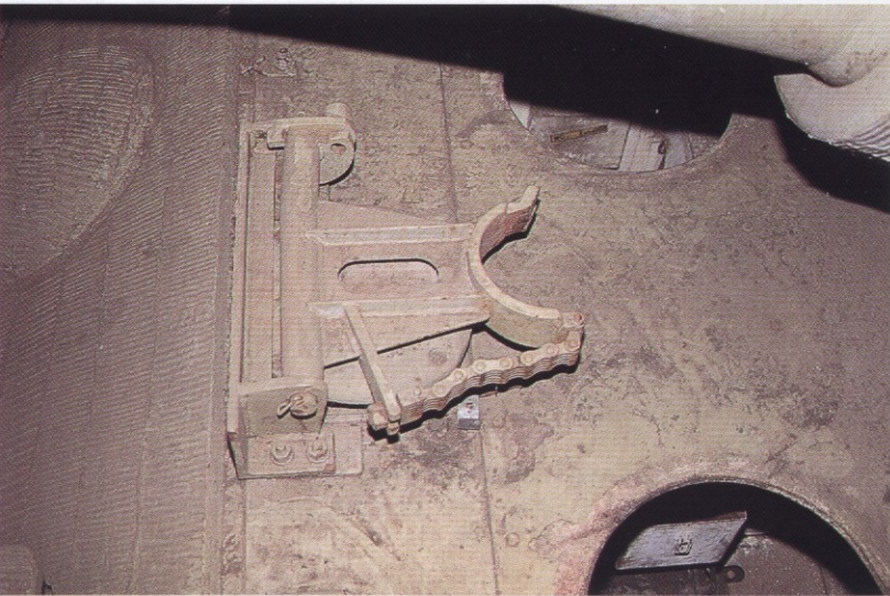
When not engaged, the lock is stowed on the armored protective cover of the hull ventilator fan.
