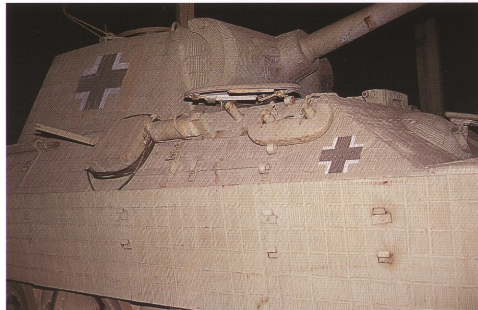
View on the frontal hull and front starboard side. Bottom hull plate is 60mm armor plate, sloped 56° from the vertical; upper hull armor plate is 80mm thick and sloped 55° from the vertical. Note the towing hooks next to the tracks.
