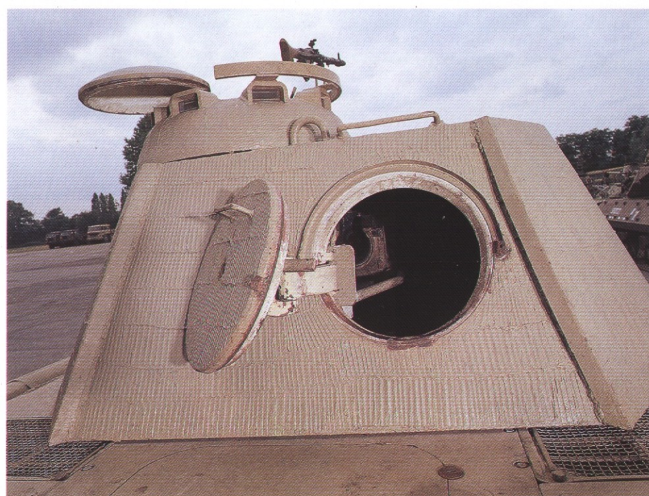
The rear turret escape hatch seen here in both open and closed position is also used for loading ammo. Similar to the sighting telescope port, the escape hatch has a rain deflection shield on the upper side. Note the 45mm armor plate on the side of the turret.
