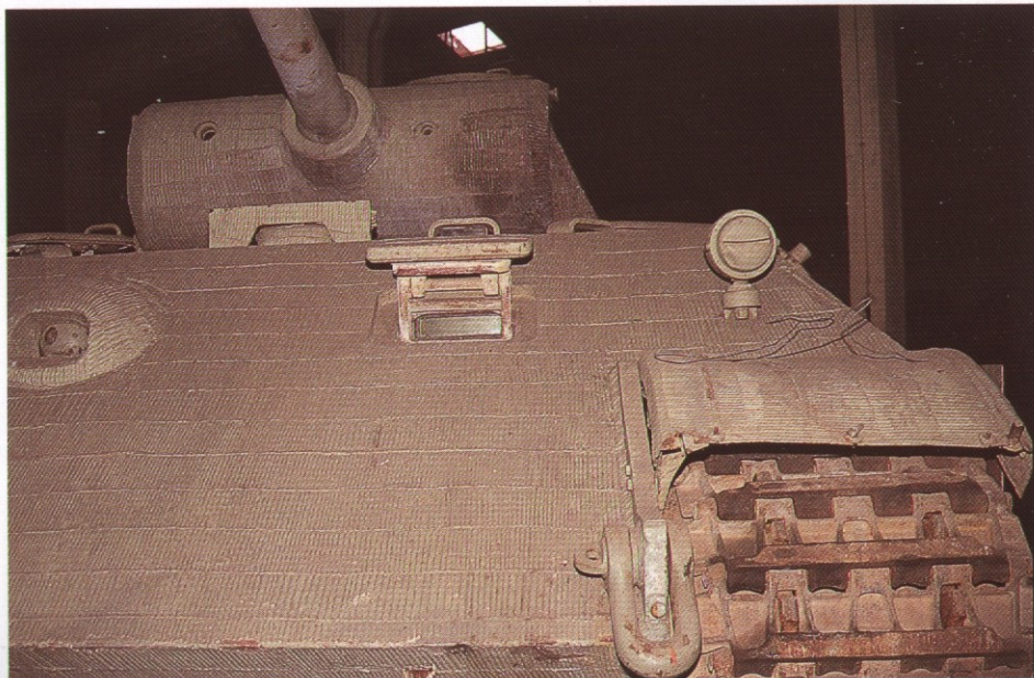
Closer look at the final drive gear housing. Note the application of the zimmeritt paste. At right can be seen the black out light, installed on port side only.
