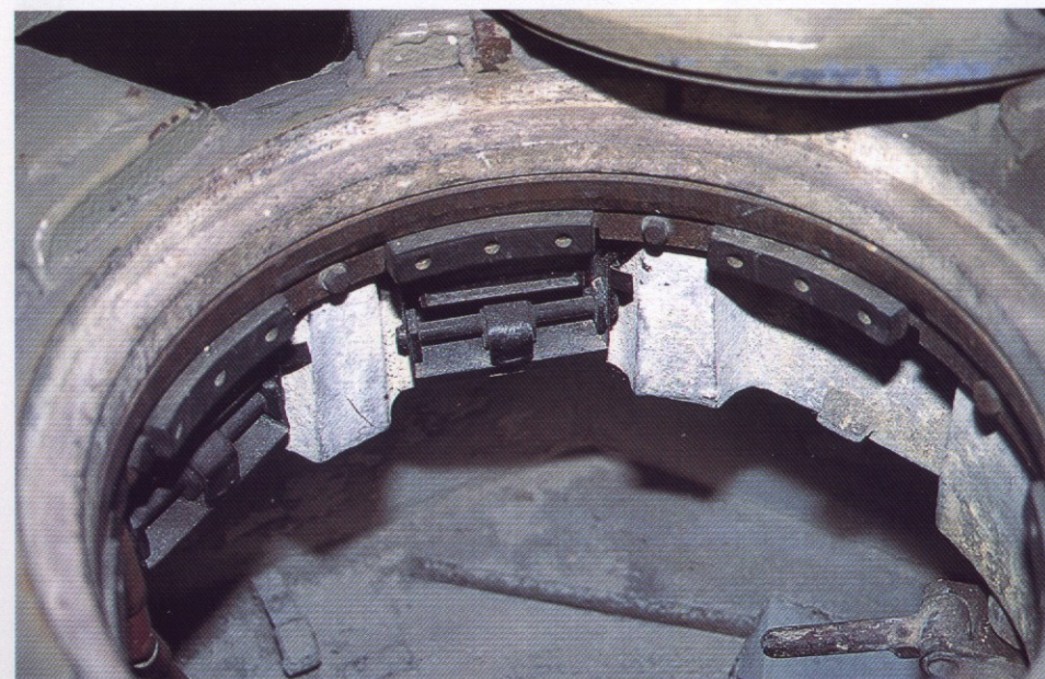
Commander's cupola featuring seven periscopes, providing 360° field of view. Note the drive shaft linkage between two persicopes.
