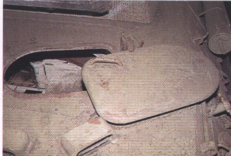
Pivoting driver's hatch in locked position. Note the periscope protective covers.
