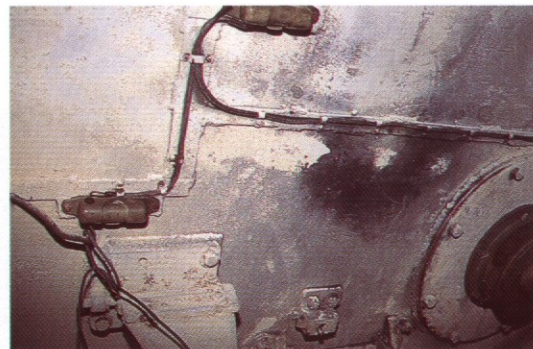
(Above) A look at some of the interior lighting domes and part of the gun sight mount at the front of the turret.
